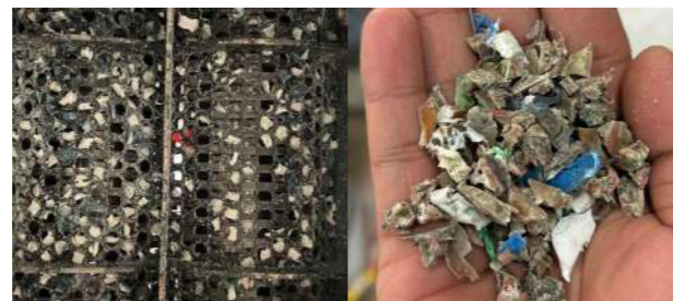
Figure 3 Sieve holes underneath the blades
