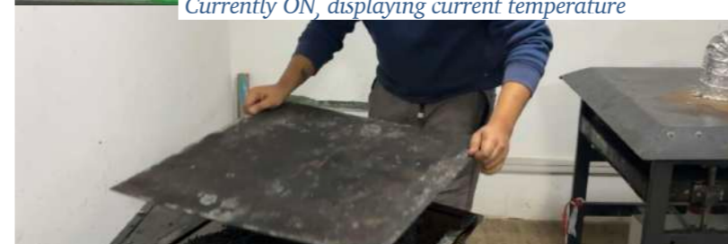
Figure 44 Layer plastic between mould and plates, add top plate
