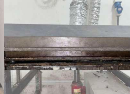
Figure 40 Heat Press (Lower the lower heating plate)
