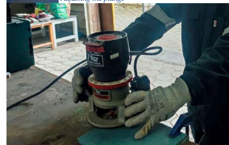
Figure 73 Routing plastic with steady pressure in proper direction
