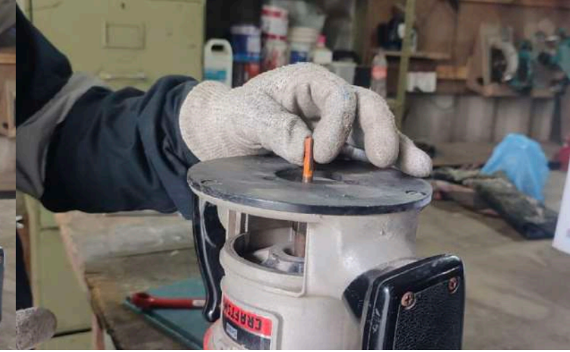
Figure 71 Adjusting the plunge
