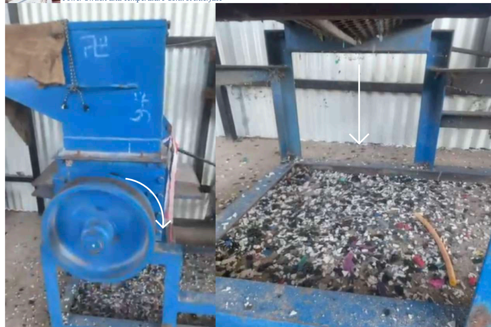
Figure 25 Grinding Chamber During Operation
