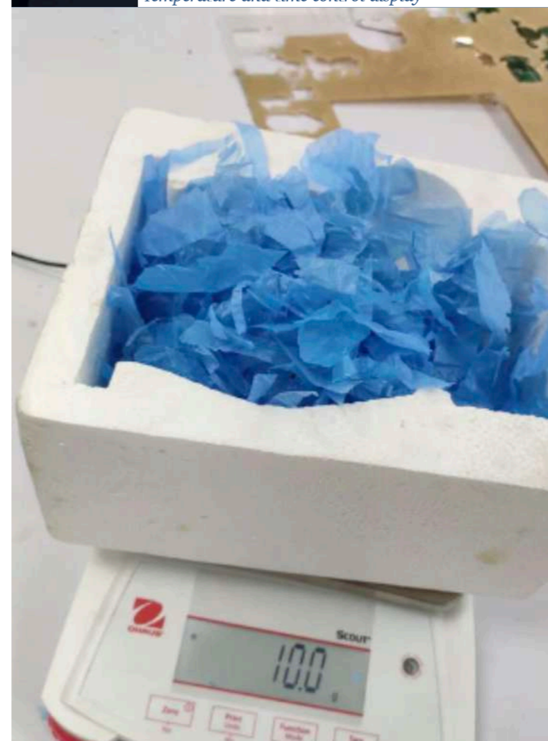
Figure 59 Measuring LDPE plastic on digital scale
