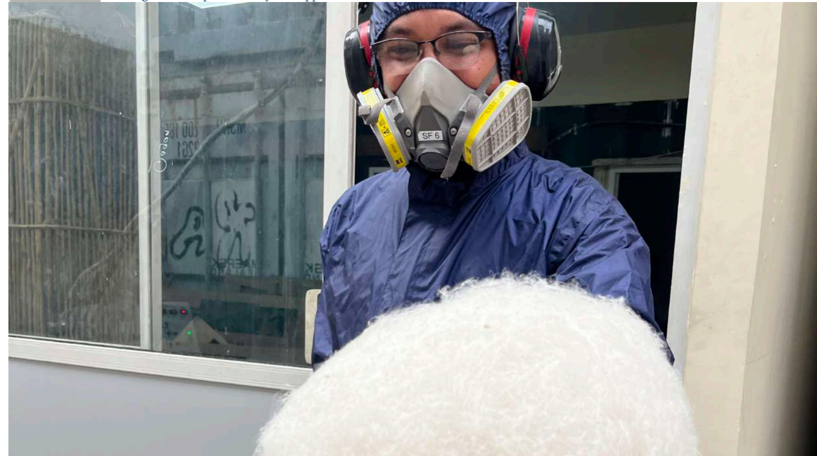
Figure 63 Removing cooled polyfloss fibres from collector compartment
