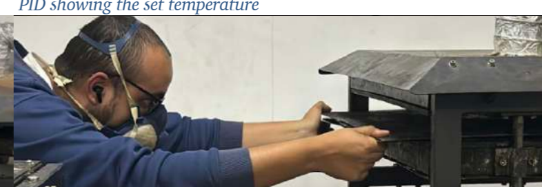
Figure 45 Place the mould on the lower plate and insert into the machine
